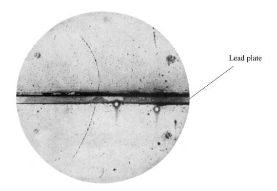
The particle was deflected by a magnetic field of magnetic flux density 1.5 T. The field is perpendicular to the plane of the photograph.
